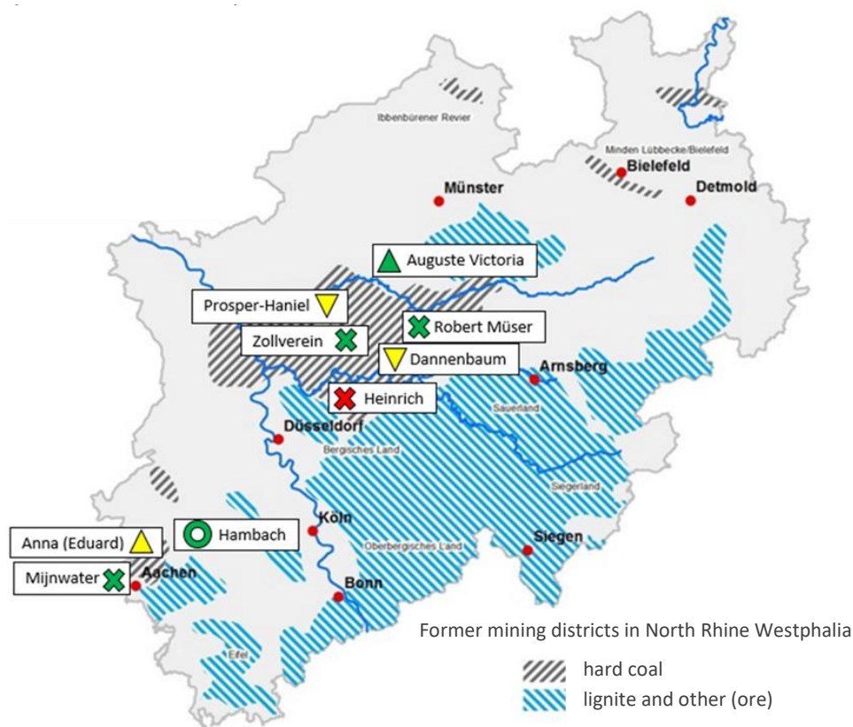
Figure 4: Project locations for mine water use in North Rhine-Westphalia and Heerlen (NL); (modified from district government of Arnsberg, 2016). Legend: - sump pit drainage, in service; - borehole heat exchanger, in planning stage; - borehole heat exchanger, in service; - heat storage, in planning stage; - mine water drainage, inoperative; - mine water drainage, in service
